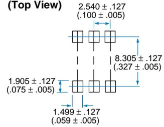
**6 Pin DIP Through Hole (Standard)**
