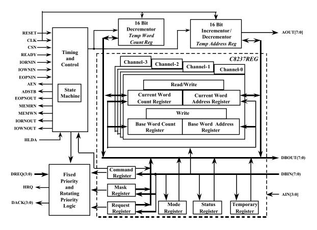
Figure 1: C8237 Programmable DMA Controller Block Diagram
