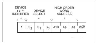
The next three bits of the slave address are an extension of the array's address and are concatenated with the eight bits of address in the word address field, providing direct access to the whole 2048 x 8 array.
