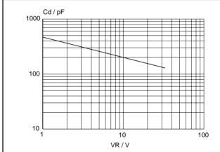
Typical junction capacitance;  $C_d = f(V_R)$ ; f = 1 MHz;  $T_j = 25^{\circ}\text{C}$  to  $125^{\circ}\text{C}$ . Fig.5.
