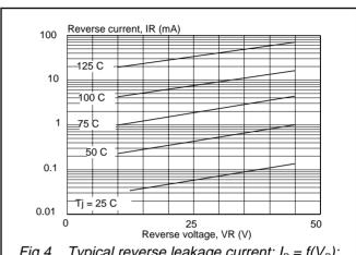
Fig.4. Typical reverse leakage current;  $I_R = f(V_R)$ ; parameter Ti
